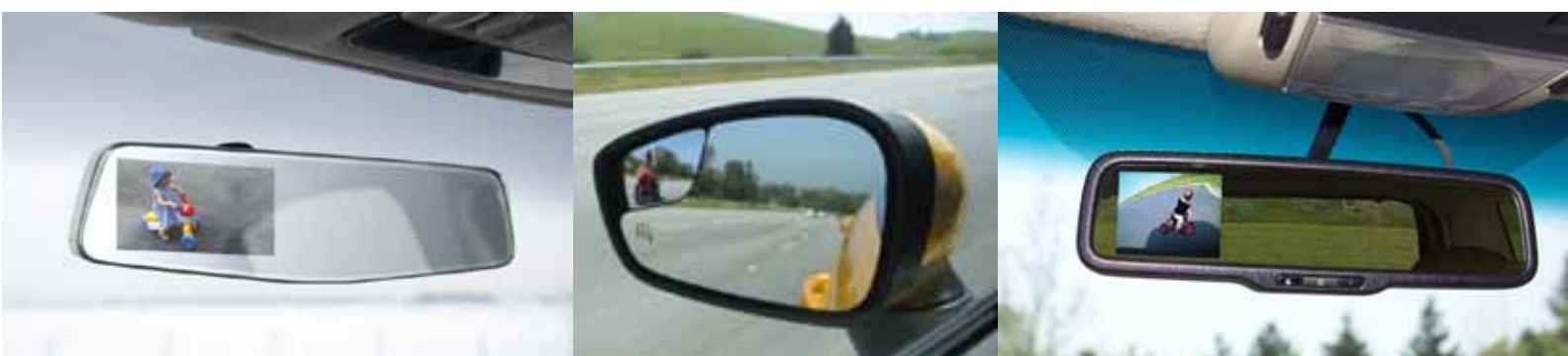
Left: Frameless Interior EC Mirror with ReverseAid™ VideoMirror™. Center: Exterior BlindZoneMirror™. Right: Interior Mirror with ReverseAid™ VideoMirror™ with Added Features.
